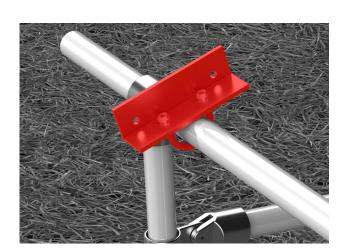
Attach U-Bolt to L-Bracket around horizontal pipe using hex nuts as shown on detail B [sheet S104].
